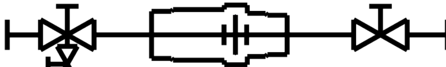
CircuitSolver Union Assembly (CSUA-W) with side drain ball valve
