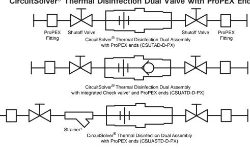
CircuitSolver® Thermal Disinfection Dual Assembly with integrated Check valve<sup>1</sup> and ProPEX ends (CSUASTD-D-PX)
