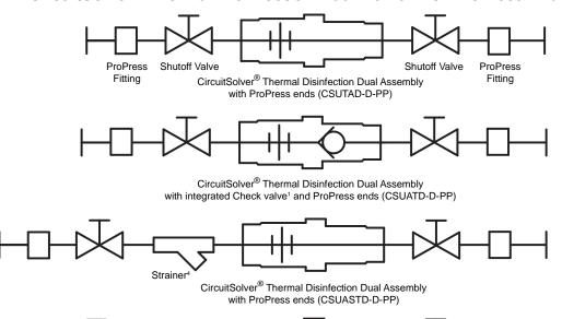
CircuitSolver® Thermal Disinfection Dual Assembly with integrated Check valve<sup>1</sup> and ProPress ends (CSUASTD-D-PP)
