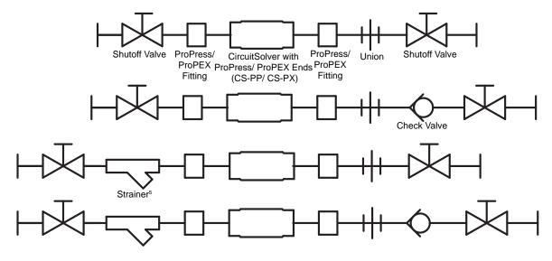
CircuitSolver® Union with ProPress/ ProPEX Ends (CSU-PP/ CSU-PX)
