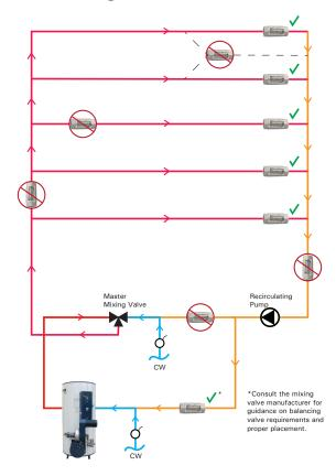
These self-actuating valves are installed at the end of each branch or riser before the return line to monitor the water temperature and will modulate open and closed to maintain a set temperature in each supply line.
