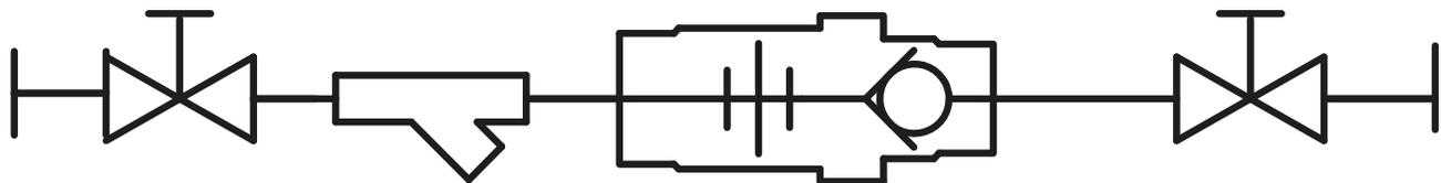
CircuitSolver Union Cold Water Assembly with integrated Strainer and check valve<sup>2</sup> (CSUAS-CW)
