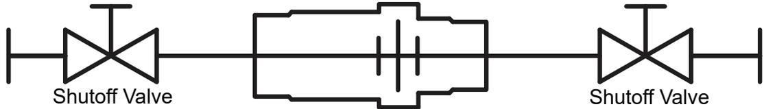
CircuitSolver Union Cold Water Assembly (CSUA-CW)
