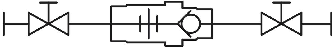
CircuitSolver Union Cold Water Assembly with integrated check valve<sup>2</sup> (CSUA-CW)
