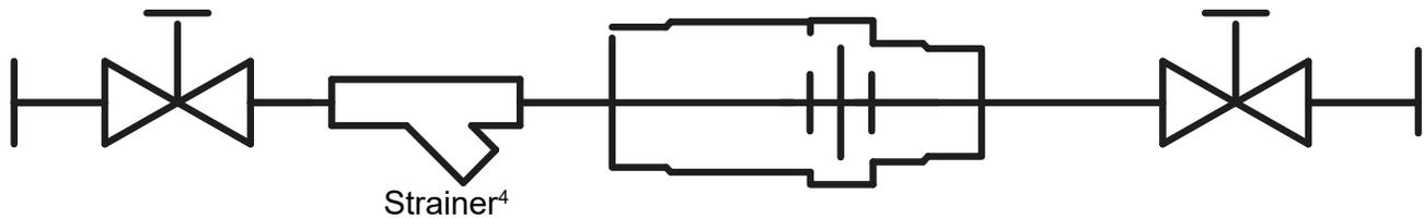
CircuitSolver Union Cold Water Assembly with integrated Strainer (CSUAS-CW)
