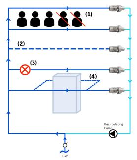
Traditional manual balancing valves could provide a solution to cold water balancing, but their static operation inherently does not factor in nor adapt to the realities of everyday system operation & changes, which may render the balancing obsolete over time.
