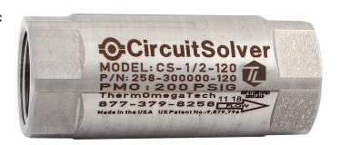
The CircuitSolver® is a thermostatic balancing valve that automatically and continuously adjusts flow through a DHW system to maintain a specified temperature at the end of each hot water supply line. This keeps the system fully balanced with hot water available at all times and on all floors, even with variable and intermittent demands.
