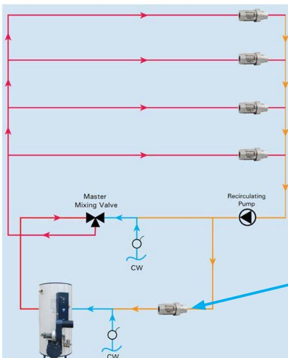
The master mixing valve output temperature is 125°F with a desired return temperature of 115°F, 10°F  $\Delta T$ .
